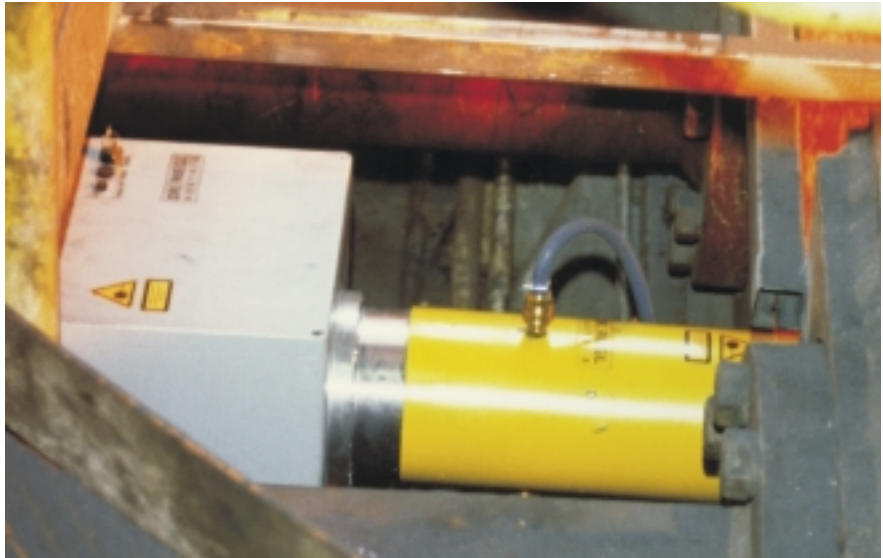
Laser distance meter LD90-2 (earlier version) with protection tube
