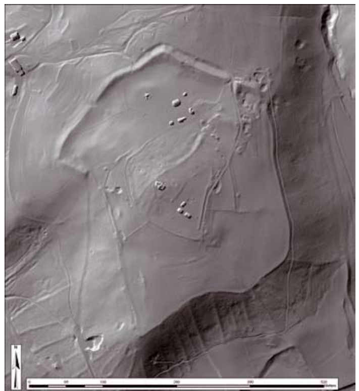
Fig. 8: Digital Terrain Model after removing all but the last echoes of the data set and filtering using the technique of robust interpolation.
