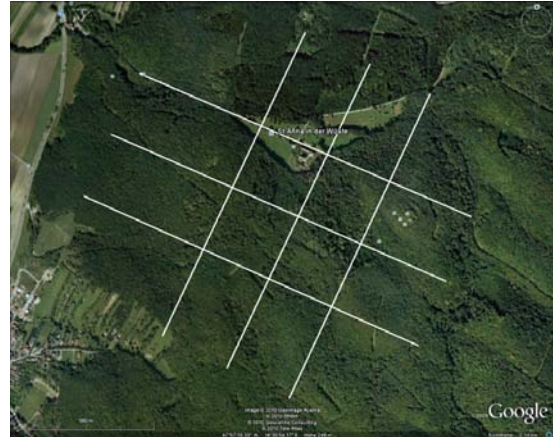
Figure 1. Study Site "St. Anna in der Wüste" in the area of the Leithagebirge (30km in the south of Vienna) with the planned flight lines (approx. length: 1.5km) for the ALS data acquisition. © Google 2010
