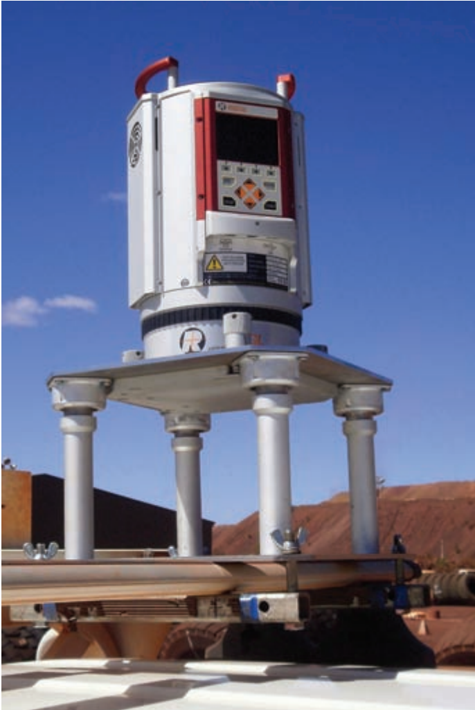
Testing the range measurement capability of the VZ-1000 at Mount Nameless (Jarndunmunha), near Tom Price Mine.
