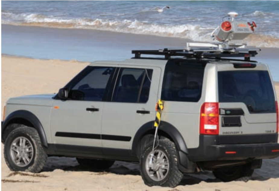
RIEGL VMX-250 Mobile Laser Scanning System: Easily mountable on the roof rack of a car
